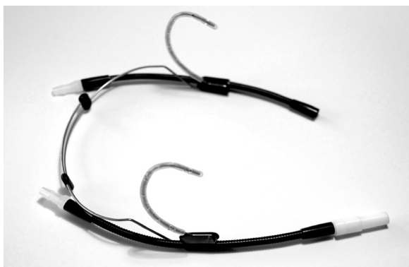
Fig. 3 Head-set for breathing-zone sampling with Mini diffusive sampler.
